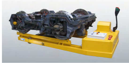
Transport vehicle: moves loads of up to 50 tons.
