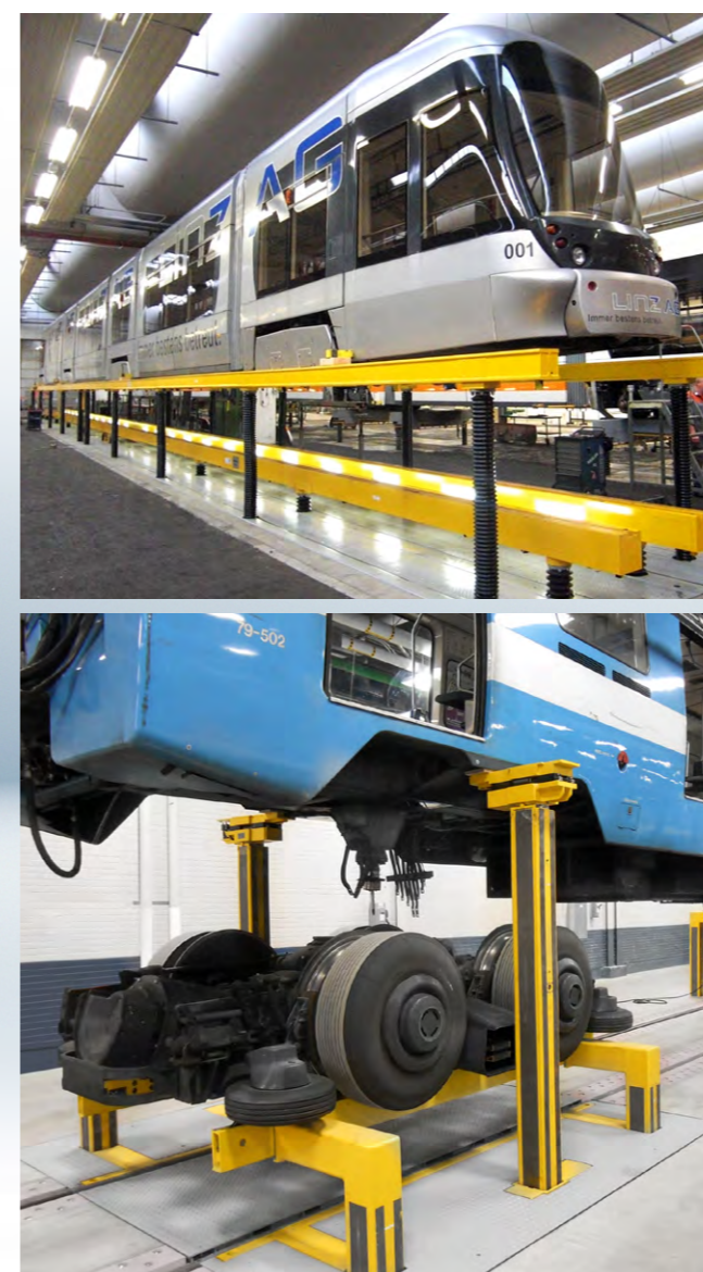
With underfloor lifting systems from Pfaff Verkehrstechnik, maintenance work can be comfortably performed on anything from trams to high-speed trains.
